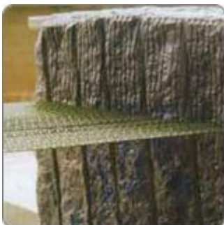
7. Granite Multi-Wires Cutting
